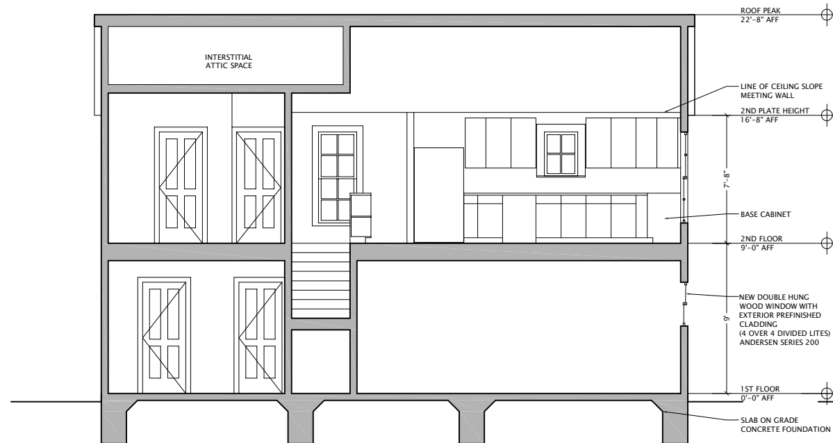
01 BUILDING SECTION SCALE 1/8" = 1'-0"
